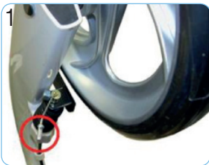
1 Remove the cable-end sleeve from brake wire.
