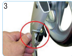
3 Loosen the cable fastener with a 4mm Allen wrench and remove.
