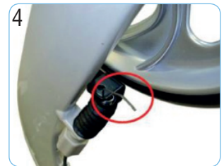
3 Loosen the cable fastener with a 4mm Allen wrench and remove.
