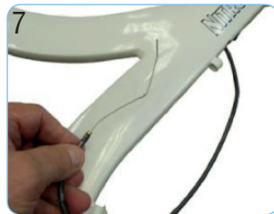
7 Tape a 5' length of cord to as much or the brake cable as possible. Do not tape the cord to the cable housing. Do not make the taped section wider than the cable housing.
