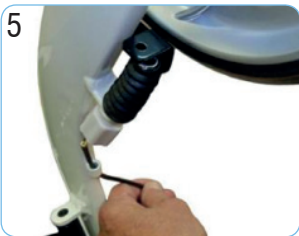
5 Remove the brake cable from the cable adjuster and spring.
