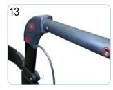
Remove the three screws holding the handle bar housing to the handle bar frame using a Phillips screw driver. Separate the two half's of the brake handle to remove them from the hand bar.
