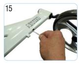
Push the new brake cable down until the brake cable can be seen in the cable hole in the bottom of the frame.
