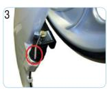
Remove the crimp fitting at the end of the brake cable.
