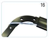
Pull the cord until the brake cable comes through the bottom of the frame.
