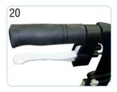
Slide the brake cable thought the two lower cable guides.
