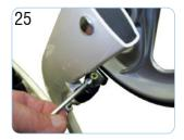
Push any excess brake cable in to the hole in the lower frame.
