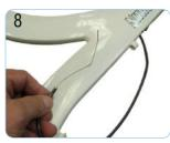
Remove the cable from the cable guides.
