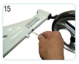
Remove the cord from the old brake and tape the cord to the cable of the new brake. Do not tape the cord to the cable housing. Do not make the taped section wider then the cable housing.
