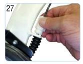
Use the cable adjuster to make any needed adjustments to the brake. If the brake can not be adjusted to engage the wheel, loosen the cable faster and reposition as needed.
