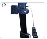
Remove the screw holding the brake handle onto the handle bar using a Phillips screw driver. Remove the brake handle.
