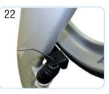
Slide the brake cable through the cable adjuster and spring.
