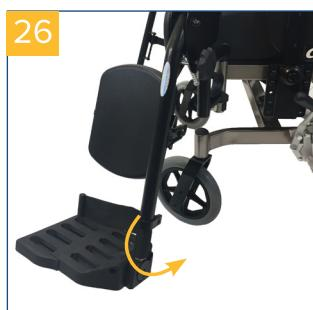
When mounting them, perform the operation in the reverse order. Ensure that the leg supports are correctly locked (pic. 26).
