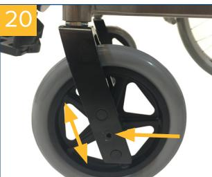
The height of the steering wheels can be changed in three steps.
