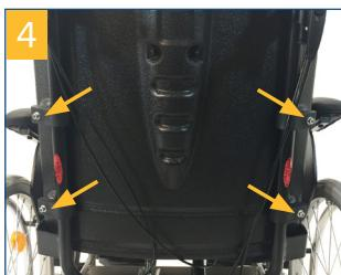
To adjust the backrest height, loosen the 4 hexagon socket screws in the retaining clips and move the backrest into the desired position, then re-tighten screws.
