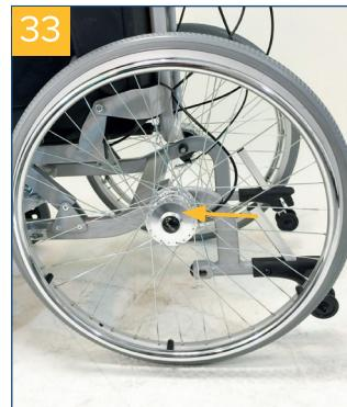
Before you take the drive wheels off, secure the wheelchair against tipping. Press on the black knob on the quick-release axle to release the connection. Then pull the drive wheel out.
